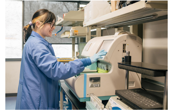
Sydney Korzep, a technician in Infectious Disease Antigen Testing at ARUP, monitors specimens in a fully automated FIT analyzer named Diana, which cuts the foil on the samples, squeezes the tubes, and checks for optical density. Diana swooshes, whirs, and occasionally beeps while testing.
